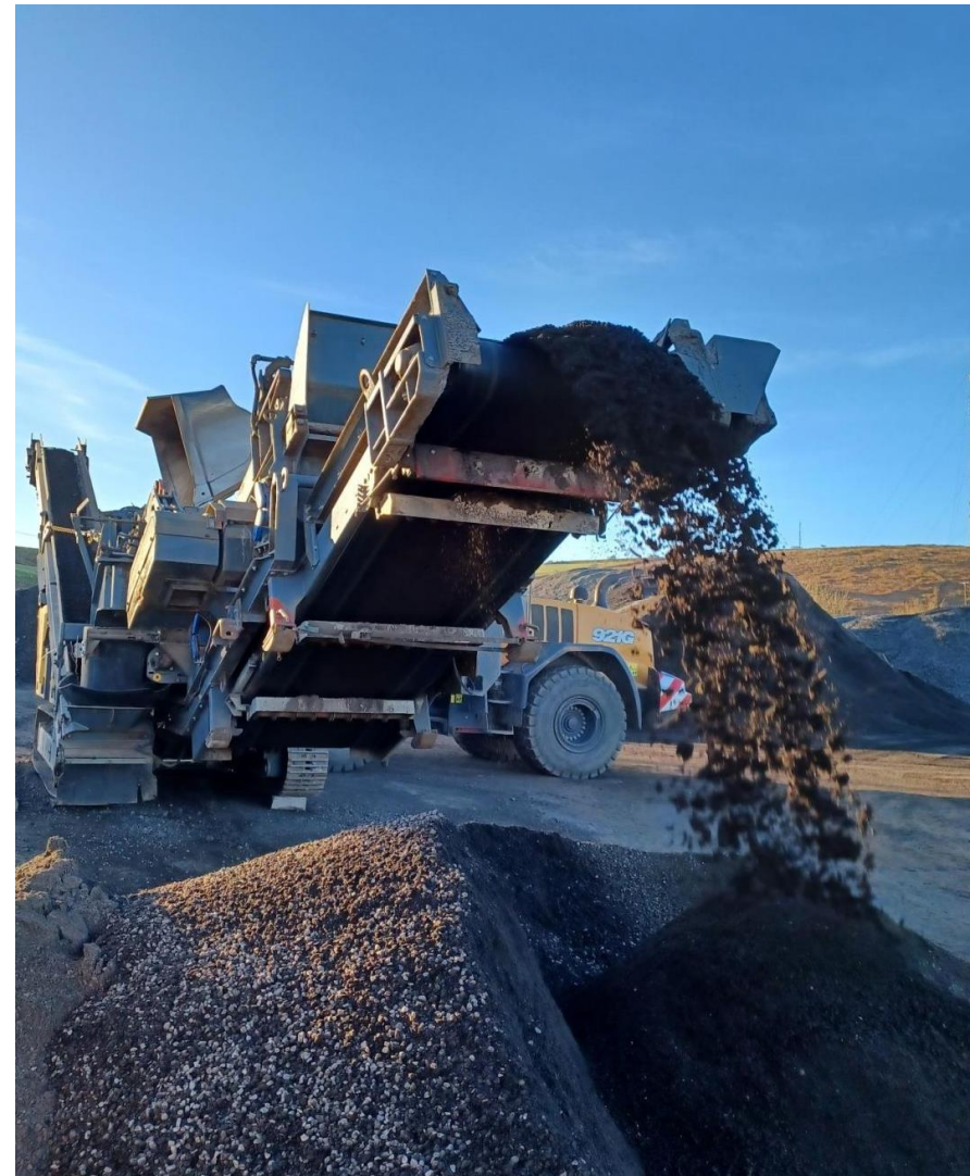
Mobile aggregate crushing and screening unit processing asphalt waste generated from maintaining Cornwall's highway network.
